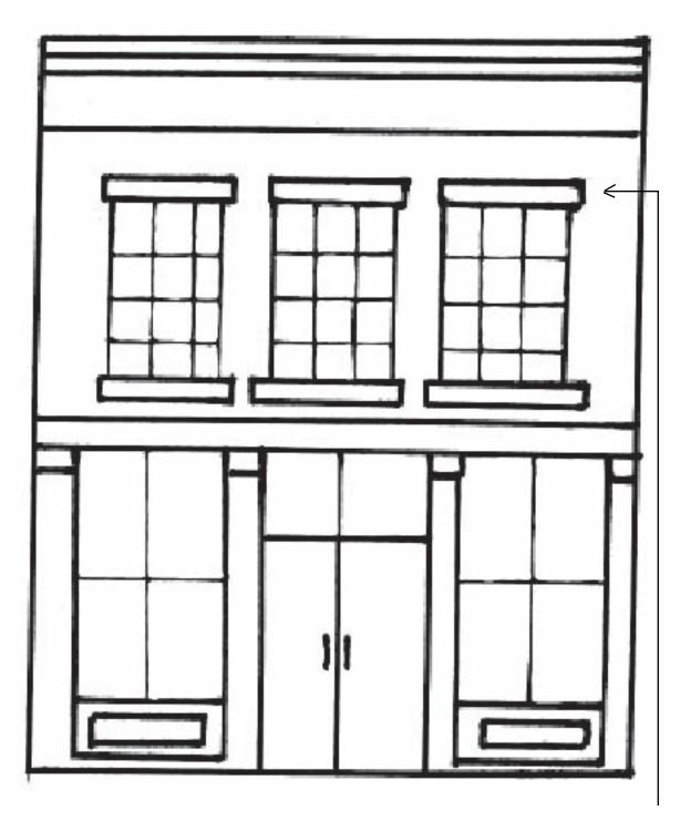
A Lintel is a horizontal structural member located above an opening such as a window.
