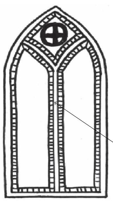
Y-Tracery is the design the mullions, or wooden slats dividing the pieces of glass in a window, form in a Gothic style window. It gets its name from the fact that the mullions are often shaped like the letter Y.
