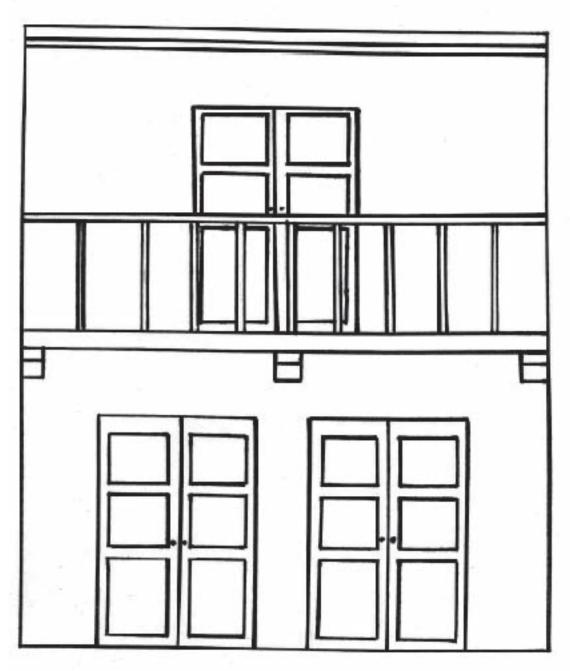
A Balcony is a platform projecting from the upper story of a building. Sometimes it is supported by posts or columns and sometimes it is supported from within.
