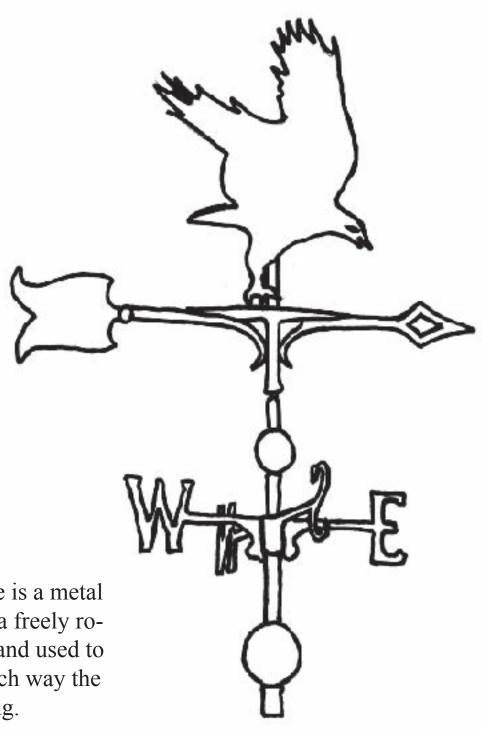
A Weathervane is a metal plate fixed on a freely rotating spindle and used to determine which way the wind is blowing.
