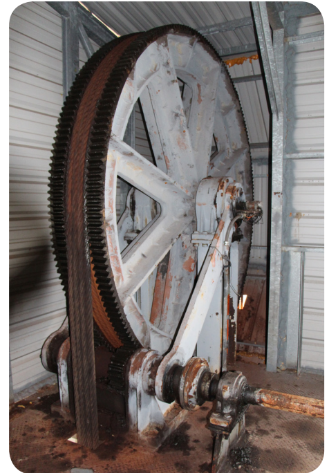
A sheave and typical drive machinery located inside the house at the top of each tower of a tower drive with independent towers vertical lift bridge (Intracoastal Waterway Bridge at Larose, Bridge Recall No. 000920).
