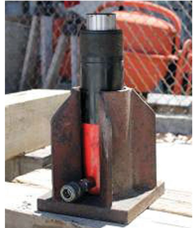
Hydraulic crib jack with adjustable base (2012)
